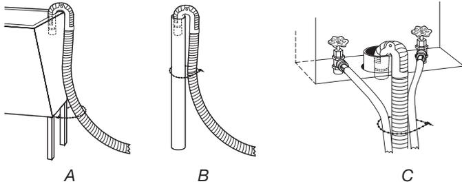
5. If the washer faucets and the drain standpipe are recessed, put the hooked end of the drain hose in the standpipe as shown. See illustration C.
